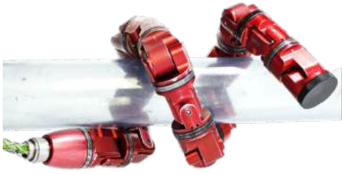
Fig. 3: A snapshot of the snake robot executing the rolling helix gait to traverse straight pipes oriented horizontally. It is described by lateral and dorsal waves which are equal in magnitude but offset by \delta = \pi/2 .
