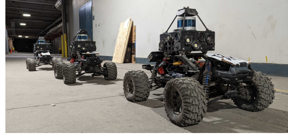
Figure 2: A multi-agent convoy consisting of three vehicles. Heterogeneous convoys are also possible using our system.
