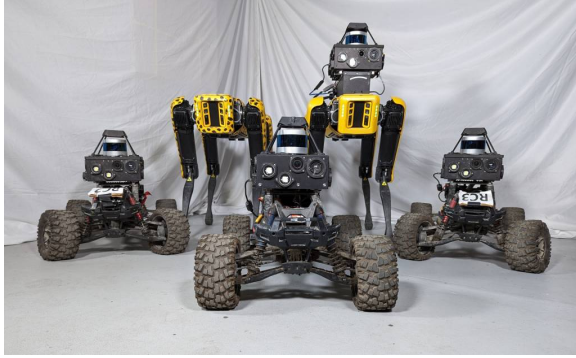
Figure 1: The team of robotic agents utilized in this work. The quadruped agents are compatible with the presented approaches but are not demonstrated herein.
